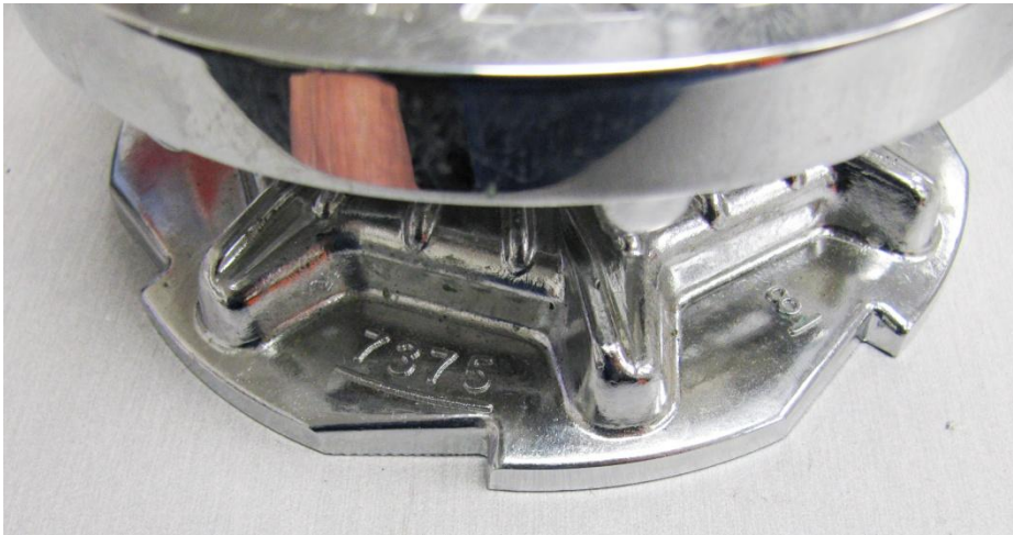
Lower Chainwheel part number location example.
