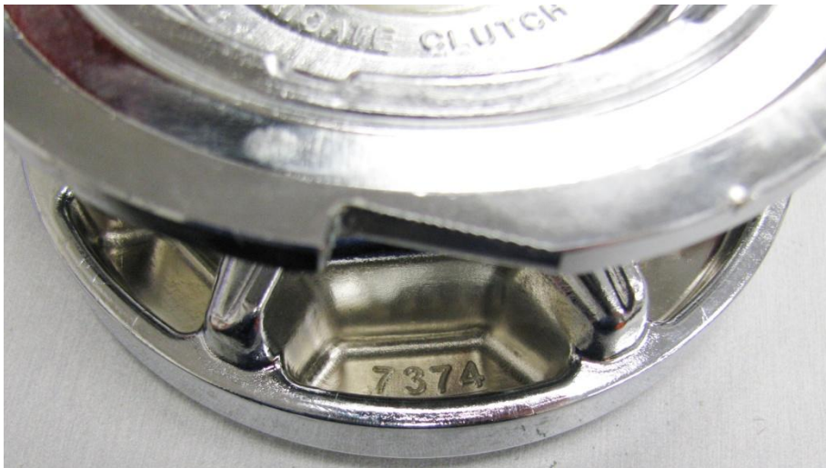
Upper Chainwheel part number location example.
