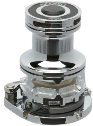
VW – Vertical Windlass Can also be mounted horizontally
